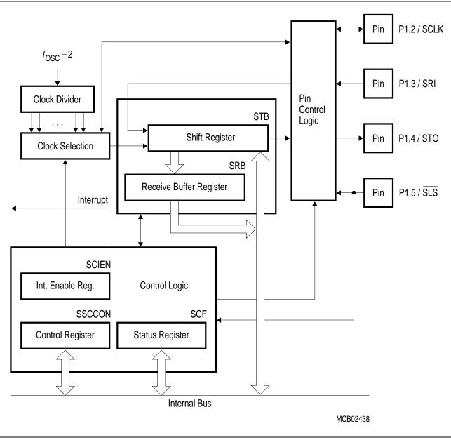
Figure 6-27 SSC Block Diagram
