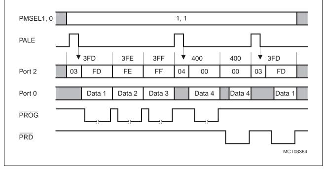
Figure 10-7 Typical OTP Memory Programming/Verify Access Waveform
