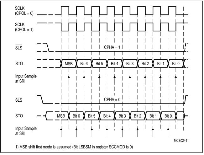
Figure 6-30 Slave Mode Operation of SSC
