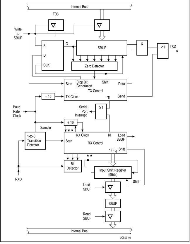
Figure 6-25 Serial Interface, Mode 2 and 3, Functional Diagram
