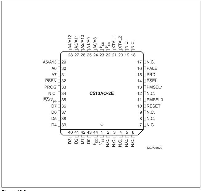
Figure 10-3 OTP Programming Mode Pin Configuration: P-LCC-44 (top view)
