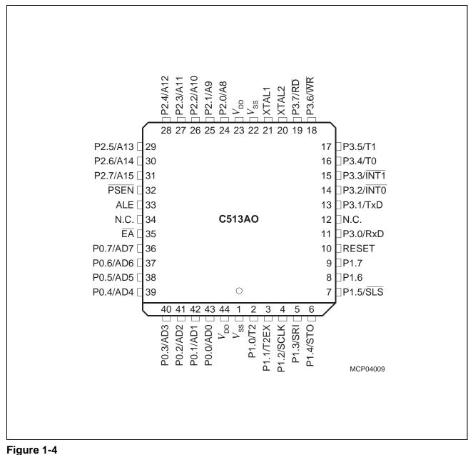
P-LCC-44 Package Pin Configuration (top view)
