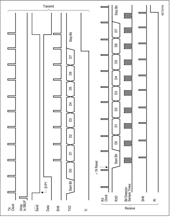
Figure 6-24 Serial Interface, Mode 1, Timing Diagram
