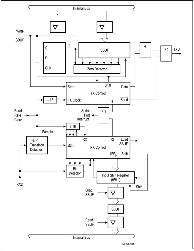
Figure 6-23 Serial Interface, Mode 1, Functional Diagram
