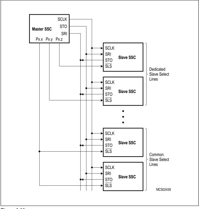
Figure 6-28 Typical SSC System Configuration
