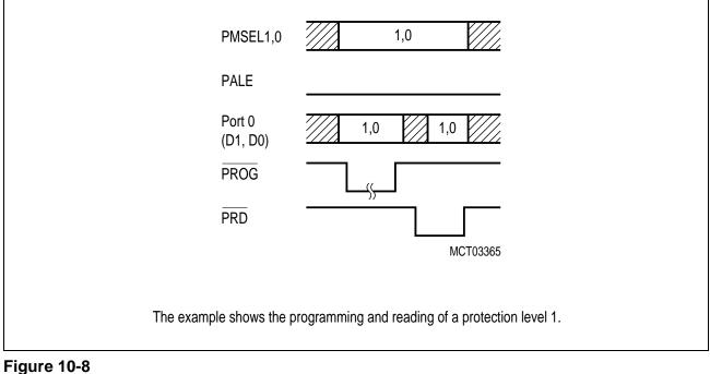
Write/Read Lock Bit Waveform
