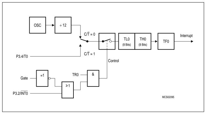
Figure 6-13 Timer/Counter 0, Mode 1: 16-Bit Timer/Counter
