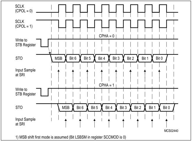
Figure 6-29 Master Mode Operation of SSC
