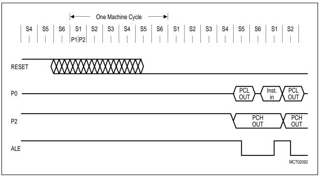
Figure 5-3 CPU Timing after Reset
