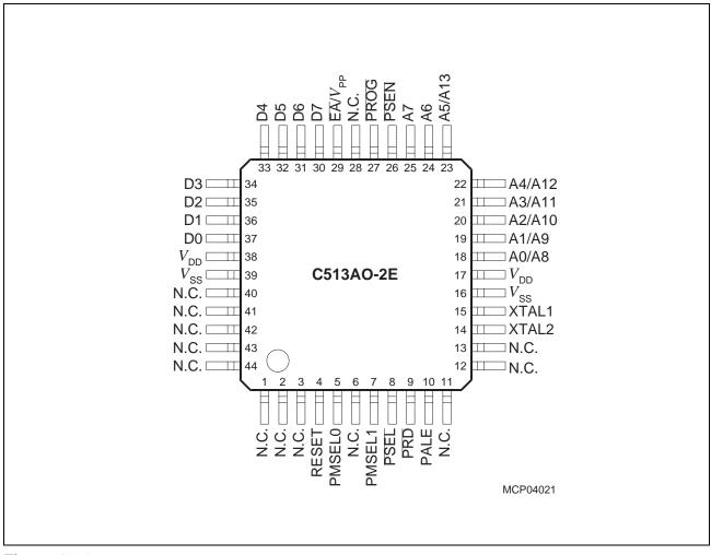
Figure 10-4 OTP Programming Mode Pin Configuration: P-MQFP-44 (top view)
