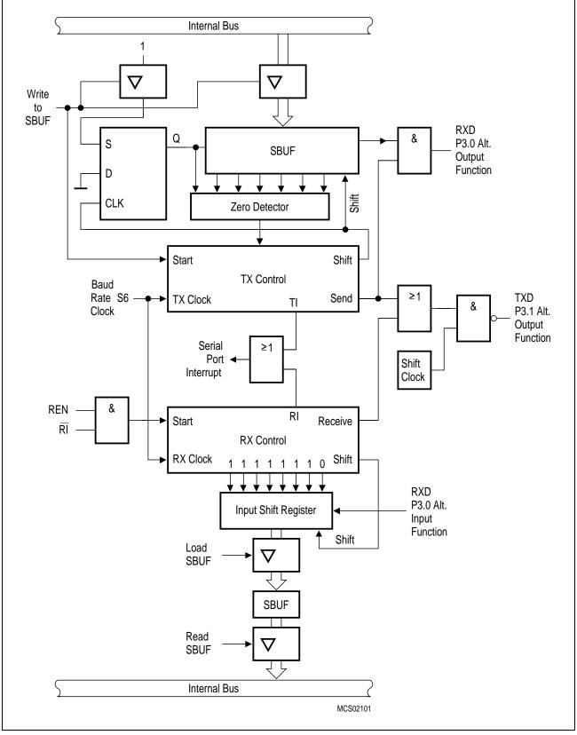
Figure 6-21 Serial Interface, Mode 0, Functional Diagram
