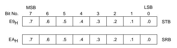
After reset, the contents of the shift register and the receive buffer register are undefined.
