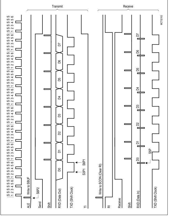
Figure 6-22 Serial Interface, Mode 0, Timing Diagram
