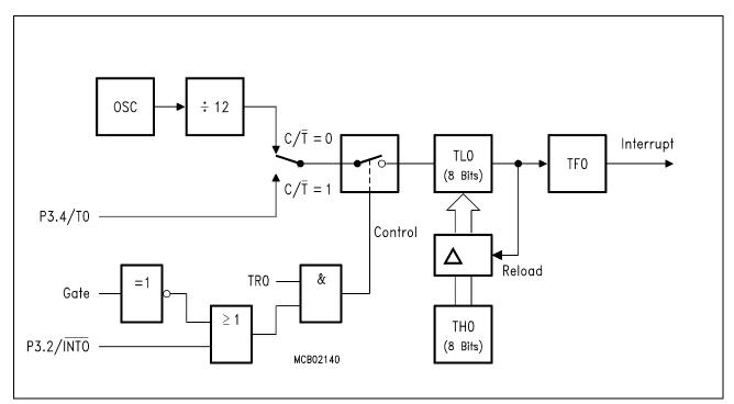
Figure 6-14 Timer/Counter 0,1, Mode 2: 8-Bit Timer/Counter with Auto-Reload
