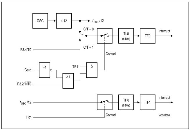
Figure 6-15 Timer/Counter 0, Mode 3: Two 8-Bit Timers/Counters
