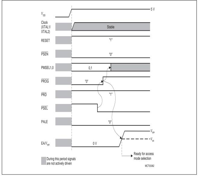
Figure 10-5 Basic Programming Mode Selection
